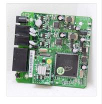
The **ATA500T** is an explosion-proof Analog/VoIP (SIP) adapter, equipped with an electronic card capable to transform an analog explosion-proof telephone in a VoIP (SIP) telephone.
