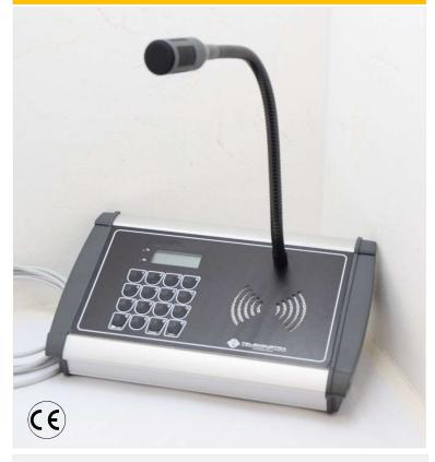
The intercom system OCEAN® is based on a "distributed intelligence". Each single intercom station is a self-standing autonomous unit, totally independent by the others. The system does not need a centralized switching unit, but a simple telephone cable (2x0,6mm) where all the stations are connected in parallel.
