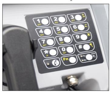
NAVY-PHONE® series "605" is a weather-proof IP66 industrial wall mounting GSM telephone, with shock-proof IK10 GRP body and heavy-duty IP66-IK10 handset, extended keypad with function keys, with protecting door. The telephone is still protected also when the door is open, because the handset and all the other devices are IP66. The door is used simply to keep clean the handset. mod. **GSM605T**
