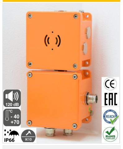
**PHONEALERT® SAP50T** is a robust weather-proof industrial **acoustic** repeater of telephone calls, designed to be installed in highly noisy areas. It is composed by two modules respectively dedicated to acoustic howler and power-supplier. The modules are made of aluminium lightalloy **IK10**, weather-proof **IP66**.
