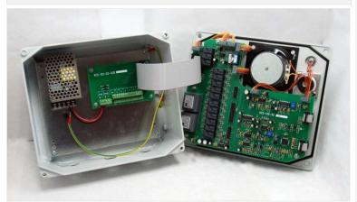
**VESSELCOM**® is a **Marine Intercom System**, designed for simple intercom networks on board of ships, **up to 10 intercom stations**. The communications channels are immediately available when you press the button relevant to the called station.
