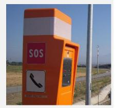
The front plate with integrated telephone can be substituted in less than a minute, **reducing the presence of maintenance personnel** in site during reparations. The lower pivoting plate, is the access to the cable terminals and auxiliary accessories area. This space is suitable for containing **auxiliary circuits** and devices (switches, power suppliers, terminals, batteries, etc.).
