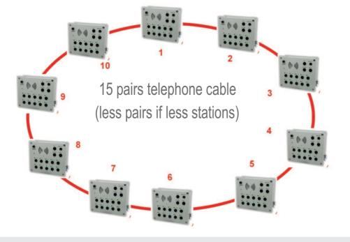
2 to 10 STATIONS **MULTI-CHANNELS GENERAL CALL** PA INTERFACE METAL BUTTONS IK10 110/230Vac and/or 24Vdc Push-to-Talk
